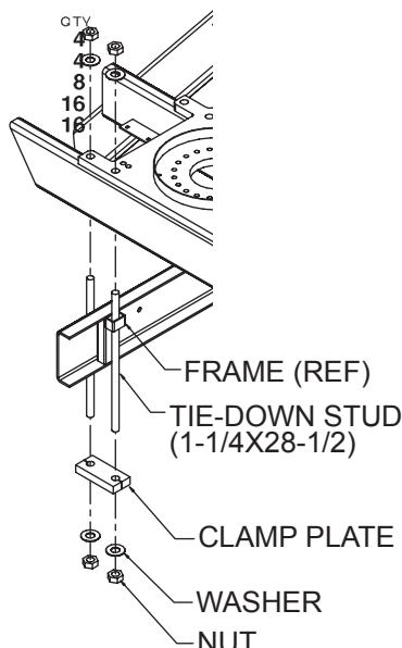
3. Allow sufficient clearance between the cab and crane base, at least 3" (7.6cm). Position the crane on the chassis per the applicable installation drawing, centering the mounting slots over the truck frame rails. While holding crane with hoist, start mounting hardware per figure below. Note position of support weldments on truck frame. Hand tighten nuts. Observe underside of crane base. No clearance between base and frame bars is allowed.
